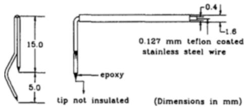
Fig. 2 Schematic diagram of two-conductivity probe
