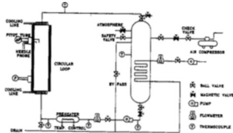
Fig. 1 Schematic diagram of test loop
