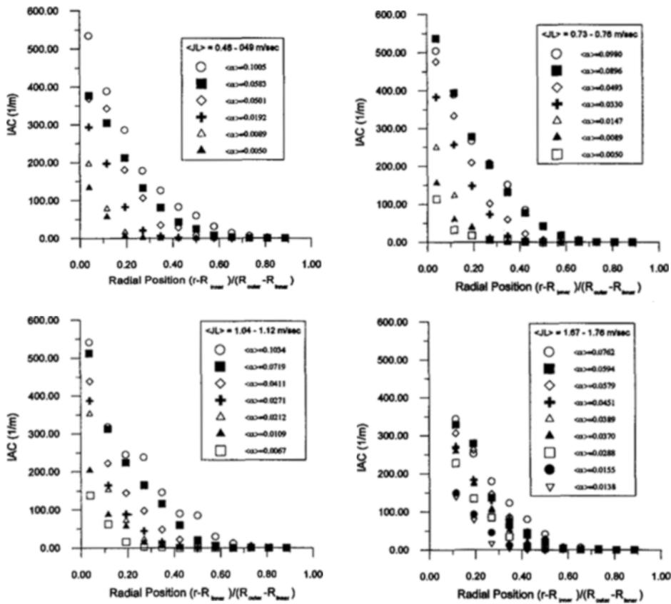
Fig. 9 Radial distributions of local interfacial area concentration in the annulus loop
