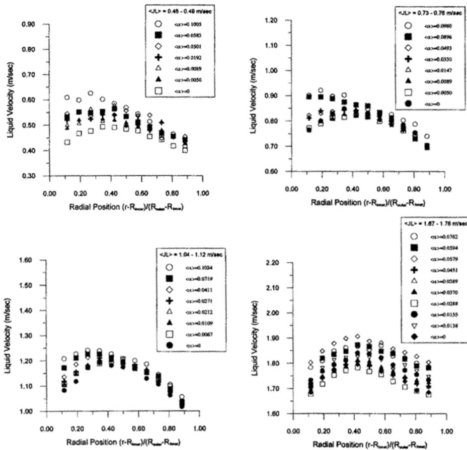
Fig. 6 Radial distributions of Local liquid velocity in the annulus loop
