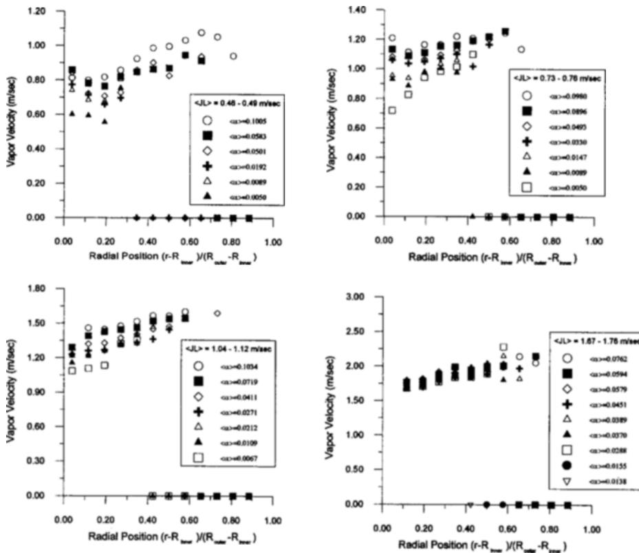
Fig. 5 Radial distributions of local vapor velocity in the annulus loop
